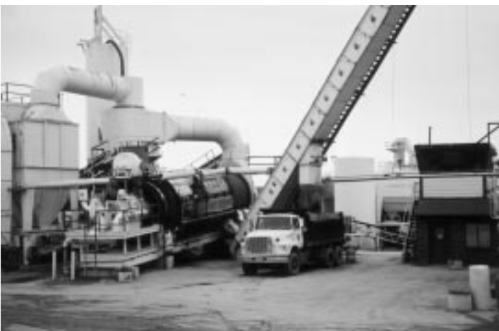
Barrett's Newtown facility uses paved surfaces for dust control and a silenced burner.
