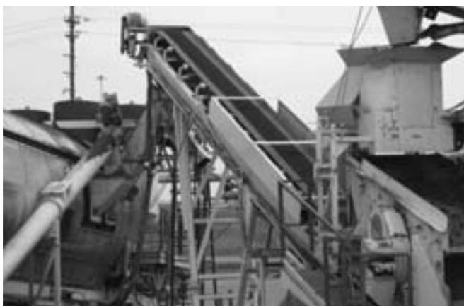
*After processing, the RAP being conveyed to the mixing drum is a very uniform product.*
