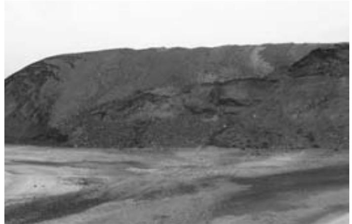
*RAP is hauled back to the HMA plant and stockpiled for processing into new HMA.*
